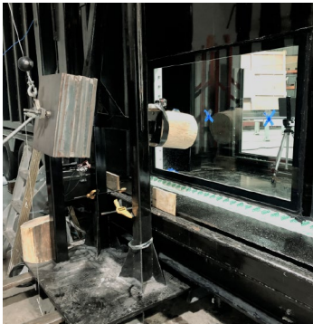
Impact Test on 4' x 6' Flood Window
