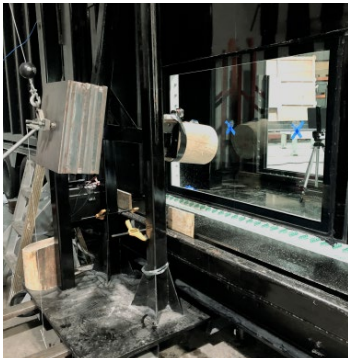
Impact Test on 4' x 6' Flood Window
