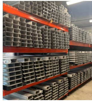
Flood log storage
