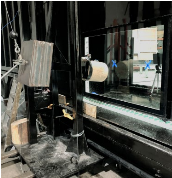
Impact Test on 4' x 6' Flood Window
