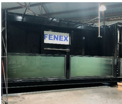
4x8' Sections Holding 4' of Water
