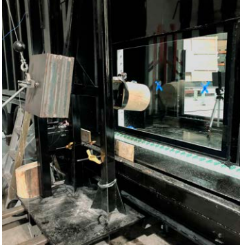
Impact Test on 4' x 6' Flood Window
